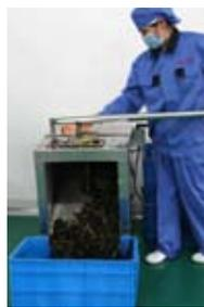
To the left, a worker is slicing Xuan Shen (*Scrophularia ningpoensis* root) on a machine that both flattens and slices herbs at the same time.
