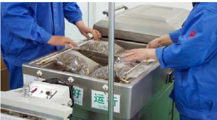
Plum Flower® herbs have two bags, the inner bag is vacuum sealed and then these bags are placed inside the outer bag that has the label on it. This outer bag is placed on another machine that both removes the regular air from between the two bags and injects nitrogen gas between them and then seals the bag. This inert gas provides two functions; it helps to reduce oxidation of the herbs and also cushions the herbs to protect them
